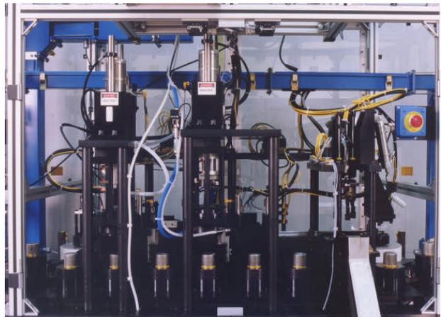
*Test-centric assemblies automatic defective parts removal*
