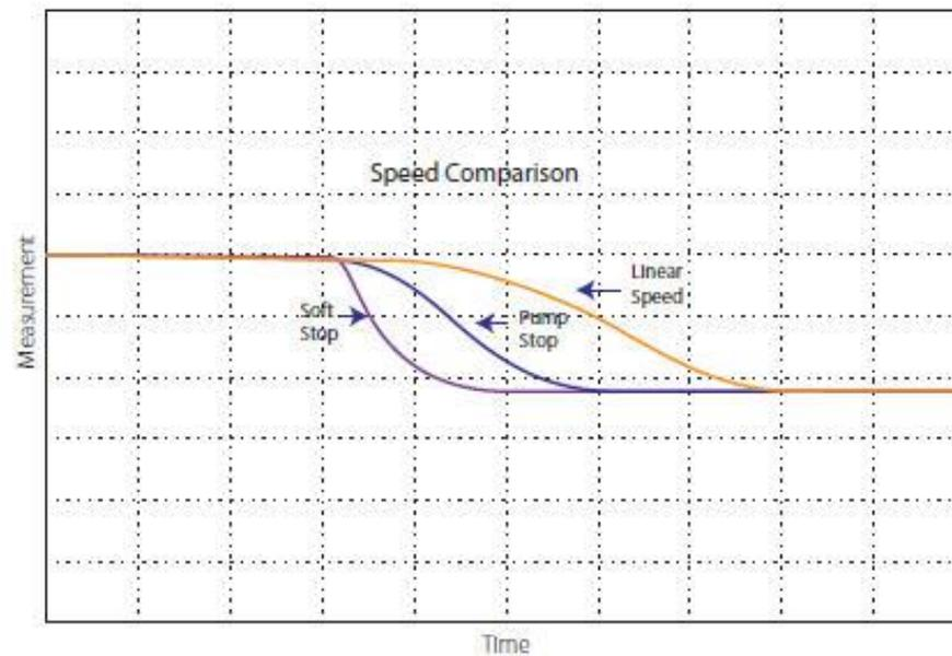
Notice the characteristics of the motor torque and motor speed when stopping. In this specific example, soft stop mode, in comparison to the motor speed, the torque drops to minimum torque at about  $\frac{1}{3}$  of the deceleration time. During pump stop, the torque drops off in approximately  $\frac{2}{3}$  the deceleration time. Linear Speed during the stop provides the most torque control for approximately  $\frac{2}{3}$  of the deceleration time.
