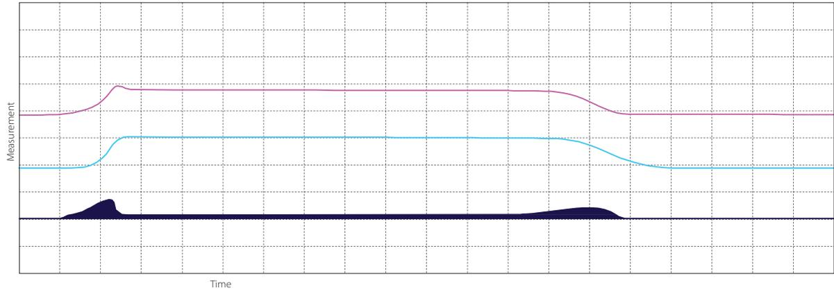
In pump start and stop mode, the motor is brought up to speed efficiently using a form of torque control that uses the algorithm and the microprocessor of the SMC-50. This enables smooth starts and stops in centrifugal pump applications, thereby reducing water hammer.
