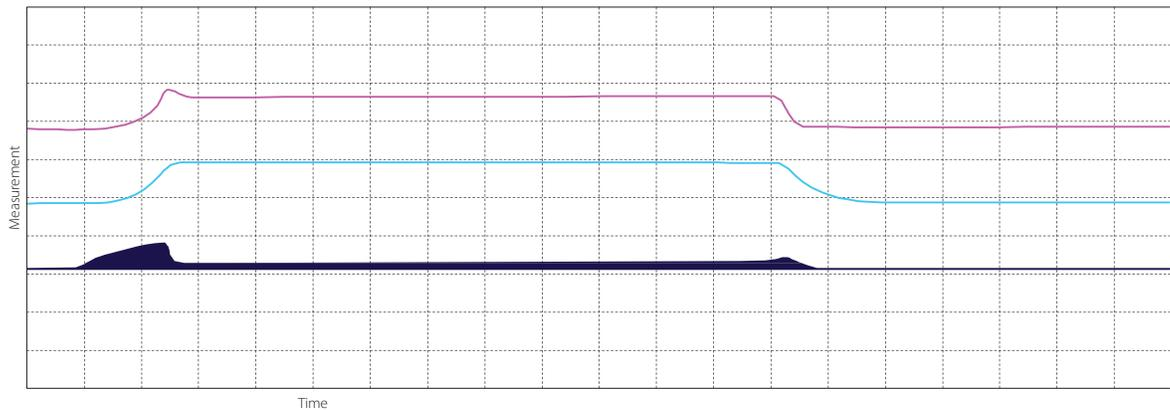
The soft start mode illustrates the current is being ramped up in proportion to the voltage ramp. Depending on system dynamics, the soft start may work fine in reducing water hammer, keeping in mind the principles of the soft start using voltage to control the start. Stopping is accomplished by linearly decelerating the voltage.
