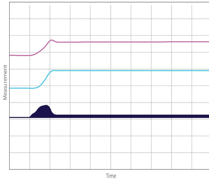
Torque start provides a solid method of bringing the pump motor up to speed with a linear torque ramp from beginning to end of the ramp. The motor speed curve will be linear when the load matches the torque profile in time.
