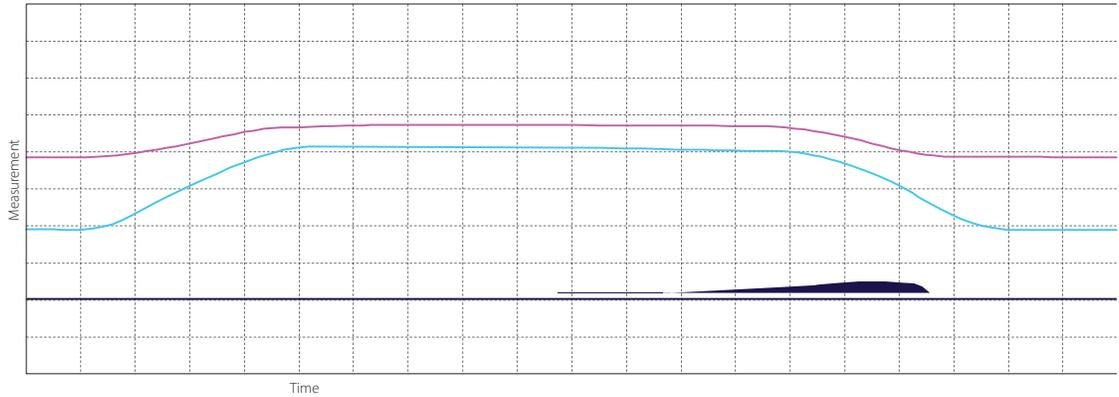
Note the smooth motor torque curve with no excessive torque. By using linear acceleration and deceleration to start and stop the pump, just enough energy is utilized to provide a smooth start and stop, regardless of the load. In stopping, you can see how long the SMC-50 controls the torque in this mode.
