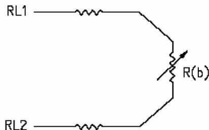
Measured resistance  $R_t = R_1 + R_2 + R_b$
