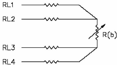
The 4-wire circuit is a true 4-wire bridge, which works by using wires 1 & 4 to power the circuit and wires 2 & 3 to read. This true bridge method will compensate for any differences in lead wire resistances.
