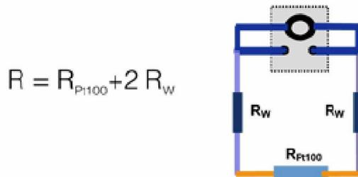
**Example 1:** Pt100 RTD 2-wire connection with direct wiring
