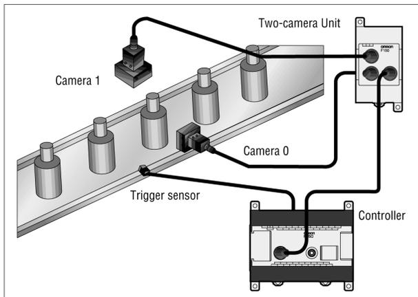
An example of a two camera sensor with separate controller—Omron's F150-3 Vision Sensor.
