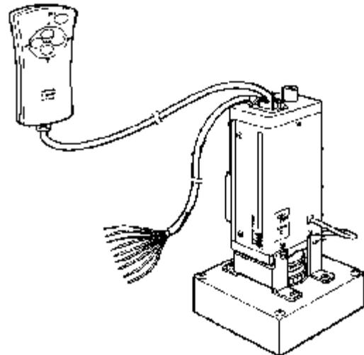
An example of a self-contained camera/processor/light source/lens--Omron's F30 Vision Sensor.
