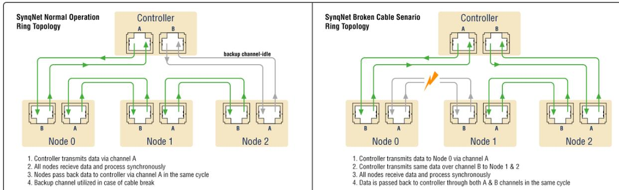
**Figure #5, SynqNet Fault Tolerant Topology**
