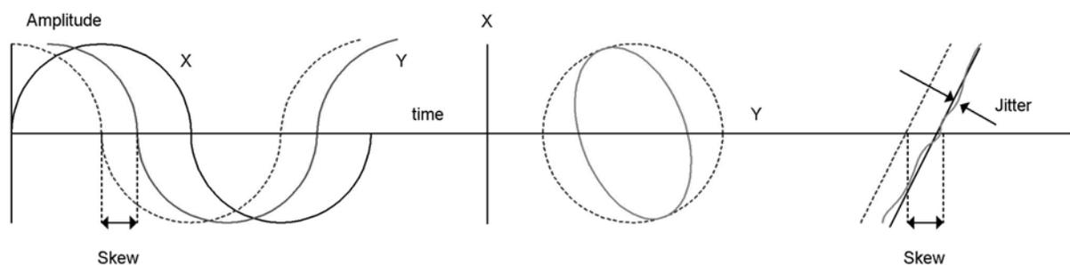
Figure #3, Effects of Jitter and Skew in Motion Control
