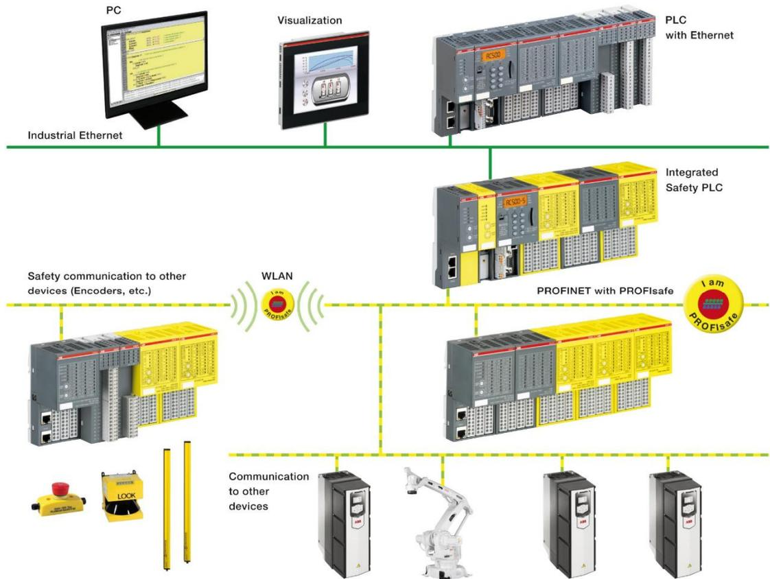
**Figure 2: Exemplary PROFINET/PROFIsafe network with advanced failure detection means in safety application program on Safety PLC**
