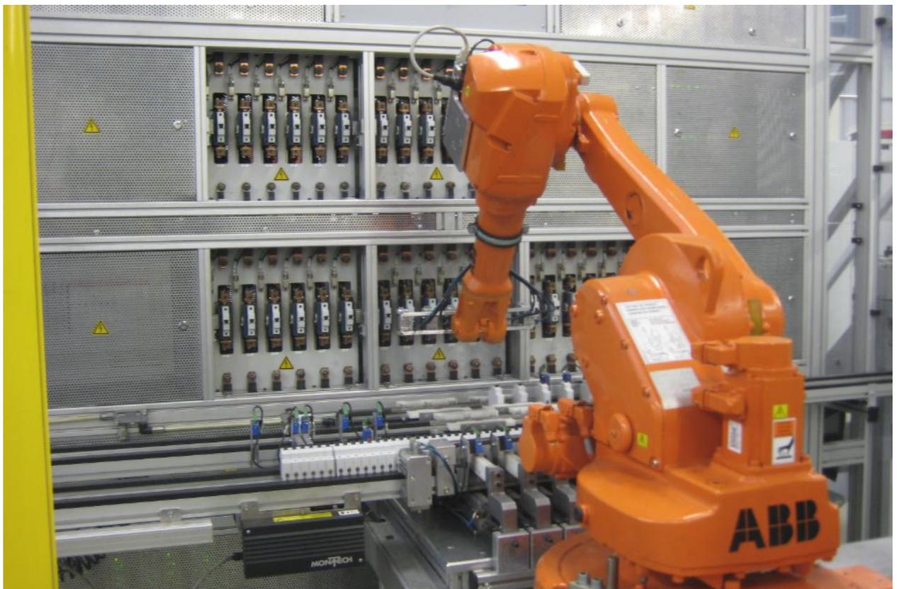
**Figure 3: Robot cell for thermal short-time measurement of MCBs at ABB STOTZ-KONTAKT production facility in Heidelberg, Germany**
