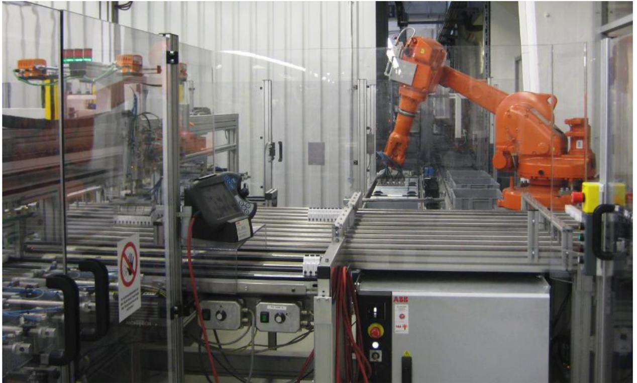
**Figure 4: Robot cell with handling of MCB poles in the storage at ABB STOTZ-KONTAKT production facility in Heidelberg, Germany**
